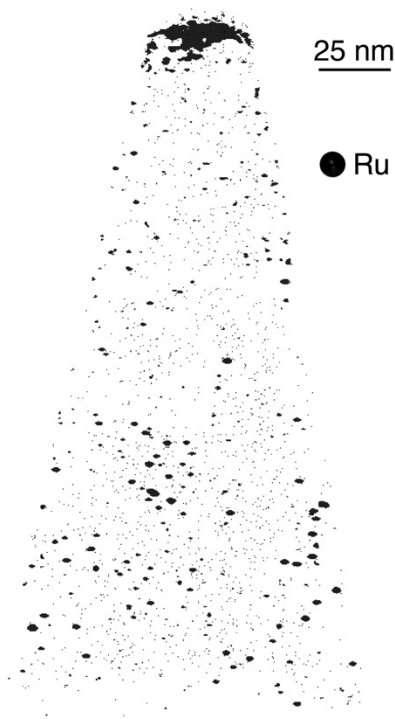
Figure S4: APT reconstruction of Ru distribution in the thin film deposited at P_{O_2} = 0.015 mtorr. Ru aggregates on surface, consistent with STEM EDS and EELS analysis.
