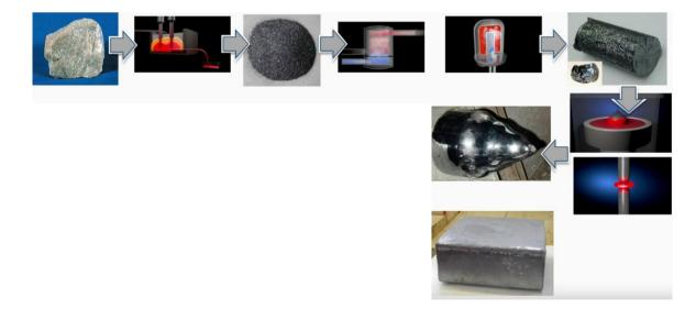
Si manufacturing is grounded in materials synthesis
