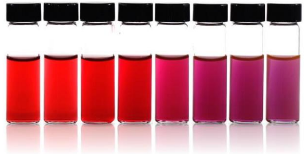
Au nanoparticles with varying plasmon resonance frequencies
